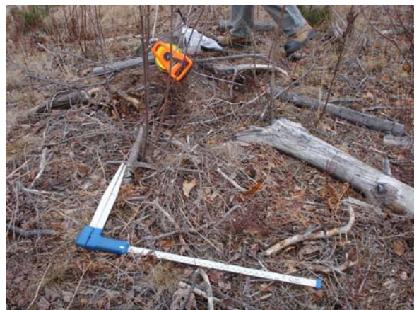
Photo: 4. Using tree calipers to lay out a 1x 1 m subplot
